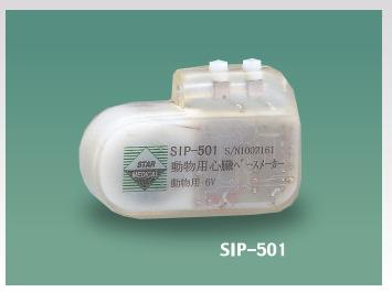
SIP-501 is the standard model of our pacemakers, with perfectly reliable waterproof covering made of epoxy resin to shut out any kind of body fluids. You can control its pulse rate externally from the outside of an animal's body with a magnet to switch the rate, from the slowest to the fastest in 9 gradual steps including OFF.
